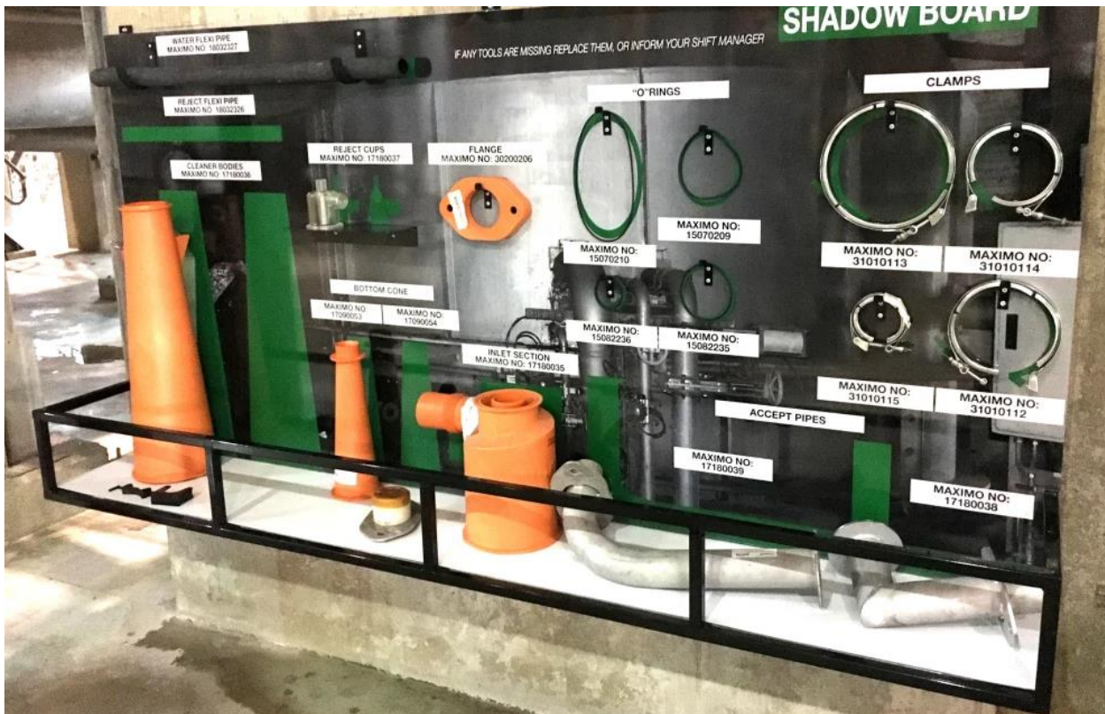
Figure 2: Example of a Shadow Board Layout for Tool Organization, illustrating a systematic arrangement of tools with clearly labelled outlines to ensure efficient and consistent tool storage in an industrial workspace.
